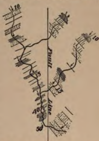
FIG. 45.—Map to show how a fault may be indicated in abrupt changes of the strike and dip of neighboring exposures.
